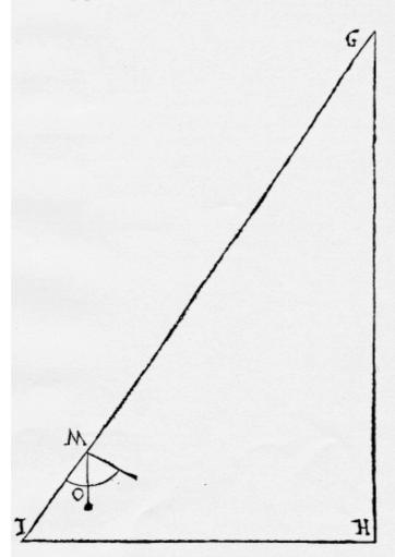
into 10,000; the result will be the number of units contained in height GH. For example if the thread cuts point 50 [in the arc near the eye], then divide 50 into 10,000 and get 200, and that many units [of which 100 equal IH] will be contained in height GH.
