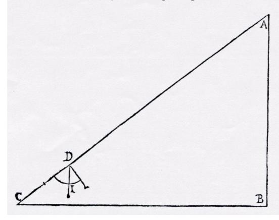
at the height A, as is seen for side CDA, and note the graduations cut by the thread DI. If these fall in the 100 away from the eye, as in the given example for arc I,<sup>22</sup> the number of those graduations is the number of paces (or other units we have measured along the ground) that we shall say are contained in height AB. But if the thread cuts the other 100, as seen in the next diagram
